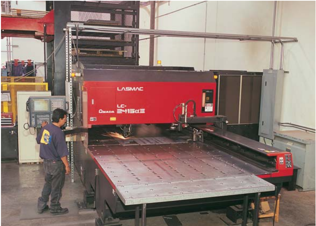
Laser operator Florentino Sierra checks on operation of Bayless' Amada 2000-watt Lasmac 2415 laser, which is equipped with a model LMP3015 6-shelf pallet loader. Because of set-up speed and large material handling capability, the laser is used for lights-out production. It is also used for prototyping and production of templates used in setup of turret punch presses.
