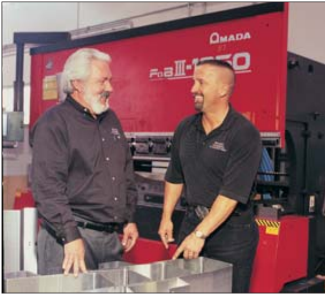
Earl Bayless and company vp Rod Smith discuss the bend radius and customer specifications for parts to be manufactured on an Amada 110-ton FBD III-3512-2004NT, 5-axis press brake. Software that drives the machine is Amada Bend Cam.
